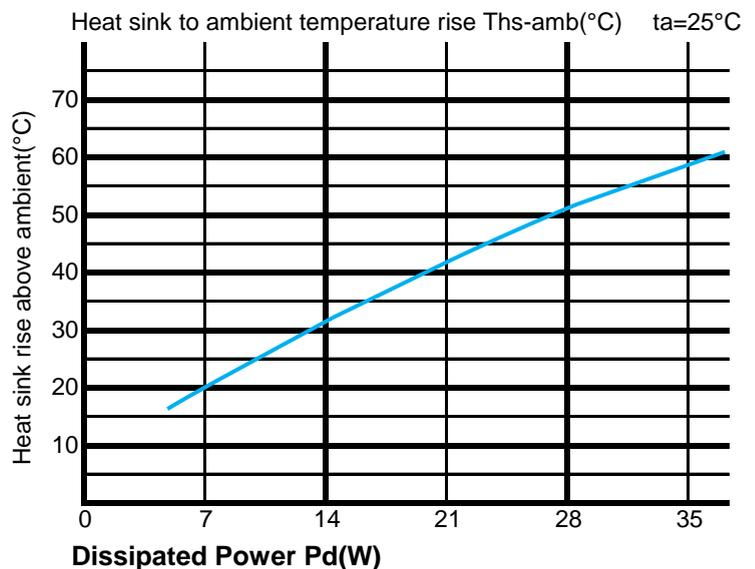
**GooLED** GooLED-86 Series  $\Phi$ 86mm Material AL1070 Pin Fin Heat Sinks Thermal Data
