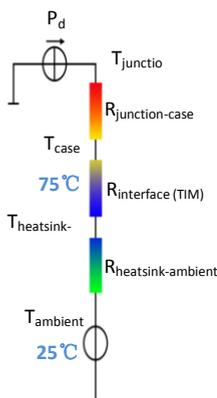
\*Thermal resistance is a heat property and a measurement of a temperature difference by which an object or material resists a heat flow.
